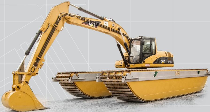
The ME-321855 is our standard model Marsh Excavator. It is typically equipped with a 20 Metric Ton / 44,092 lb. Excavator.
